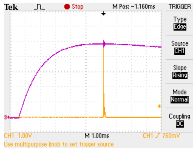
Figure B-6: Magnetic Field Coil Shunt Resistor Voltage vs. Time Curve for 60 Volt Magnetic Field
