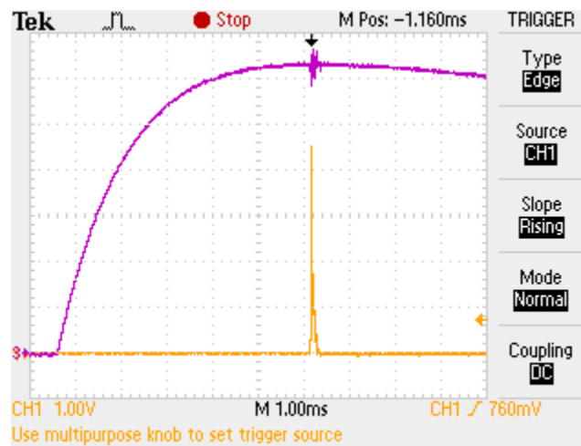
Figure B-4: Magnetic Field Coil Shunt Resistor Voltage vs. Time Curve for 40 Volt Magnetic Field
