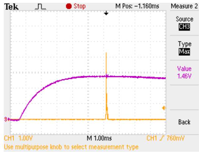
Figure B-9: Magnetic Field Coil Shunt Resistor Voltage vs. Time Curve for 90 Volt Magnetic Field
