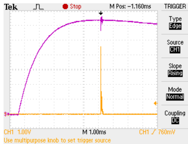
Figure B-8: Magnetic Field Coil Shunt Resistor Voltage vs. Time Curve for 80 Volt Magnetic Field
