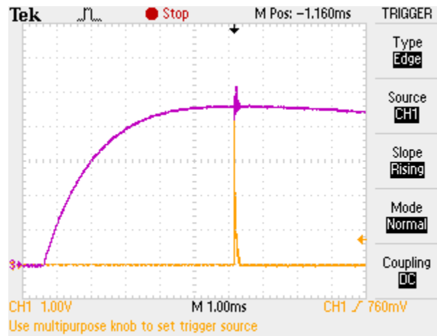
Figure B-3: Magnetic Field Coil Shunt Resistor Voltage vs. Time Curve for 30 Volt Magnetic Field
